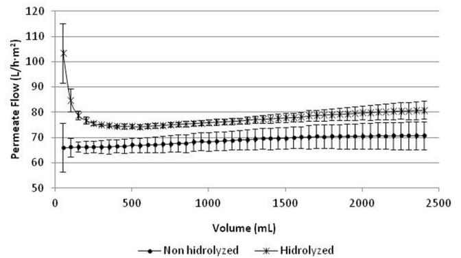
**Figure 6.** Permeate flux of hydrolyzed and non hydrolyzed cagaita pulp in tubular membrane of polyethersulfone ( $0.3 \mu\text{m}$ ) at 0.5 bar.
