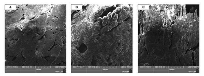
**Figure 3**. Scanning electron micrographs (SEM) of the different ultrasound times; (A) without ultrasound application; (B) 5 minutes of ultrasound; (C) 10 minutes of ultrasound.
