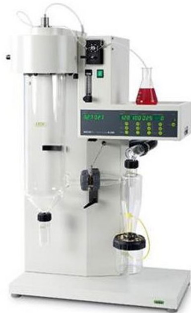
Figure 3. Dehydration scheme by spray drying and mini spray drying apparatus, Büchi, B-290. Source: Dryer Büchi (2021).
