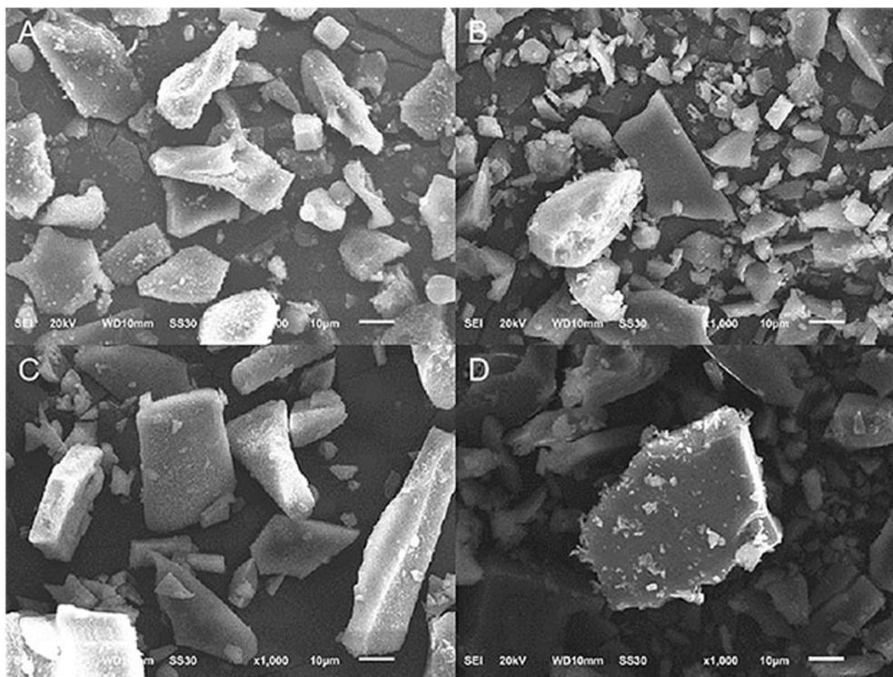
**Figure 2.** SEM images of (A) DB (B) DBH-P (C) DBH-T (D) DBH-A with 1000 times magnification.
