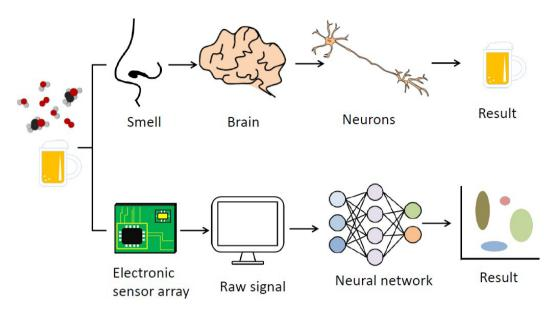
Figure 2. Scheme of the working principle of E-noses.
