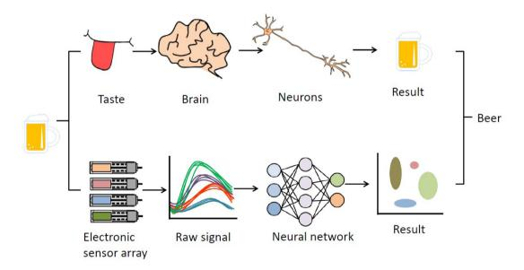
Figure 3. Scheme of the working principle of E-tongues.
