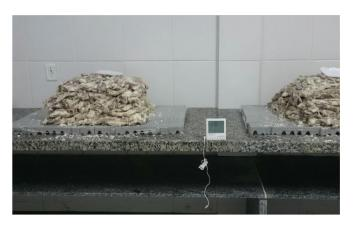
Figure 3. Pile of meat pork salting with temperature and humidity control.
