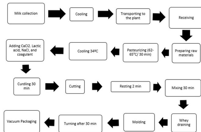
**Figure 1.** Flowchart of the cheese production process. Source: the author, according to the information from the producer (2021), adapted by Venturini et al. (2007).
