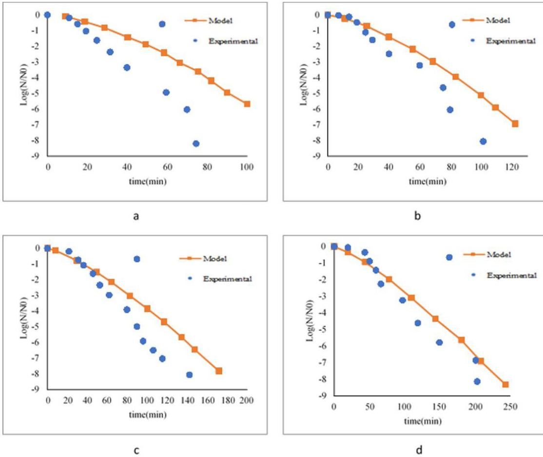
**Figure 4.** Prediction of *Salmonella typhimurium* inactivation curve in broth medium with the supercritical fluid process at 35 °C by Weibull model at pressures of (a) 7.56 MPa, (b) 6.05 MPa, (c) 3.02 MPa, (d) 1.51 MPa.
