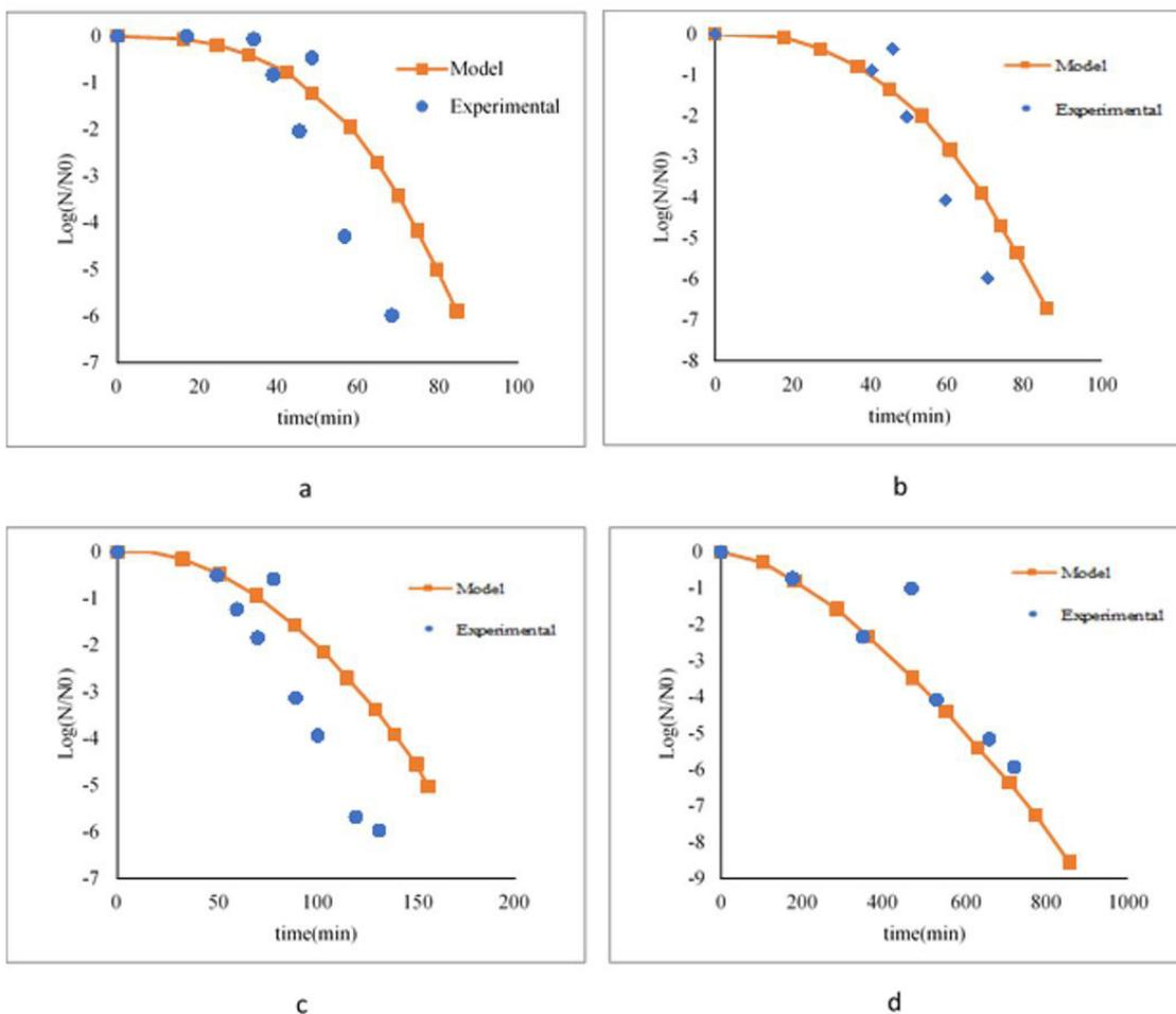
**Figure 2.** *Saccharomyces cerevisiae* inactivation curve using a high-pressure supercritical fluid with Weibull model at 40 °C and pressures (a) 10 MPa, (b) 7.5 MPa, (c) 5 MPa, (d) 2.5 MPa.
