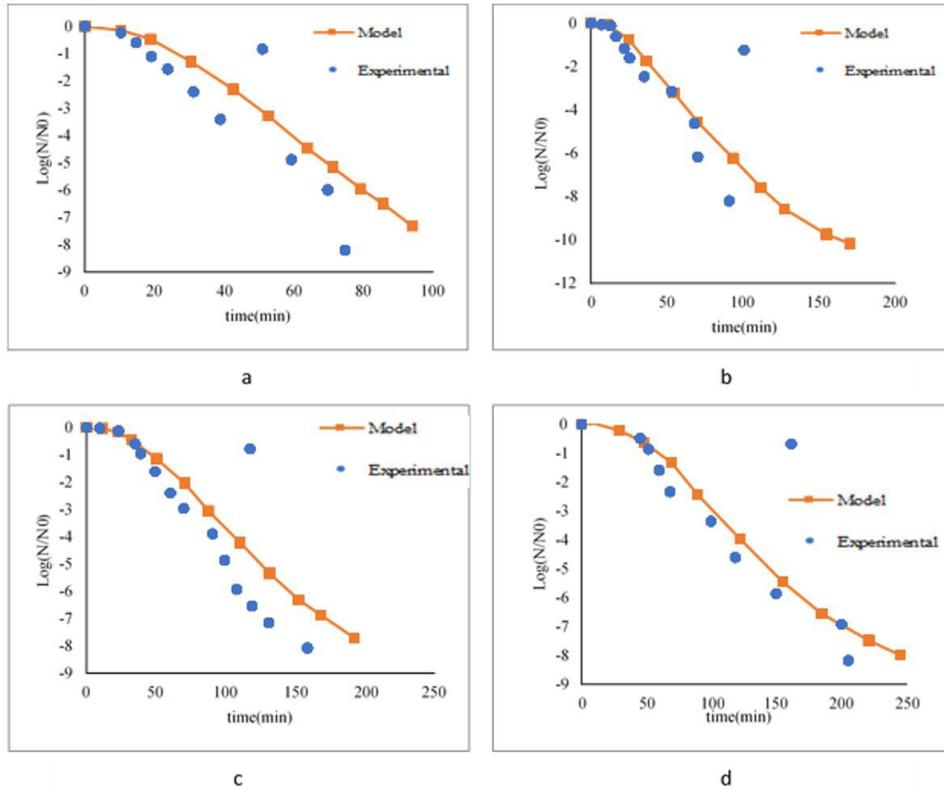
**Figure 7.** Prediction of *Salmonella typhimurium* inactivation curve in broth medium with the supercritical fluid process at high pressure at 45 °C by the log-logistic model at pressures of (a) 7.56 MPa, (b) 6.05 MPa, (c) 3.02 MPa, (d) 1.51 MPa.
