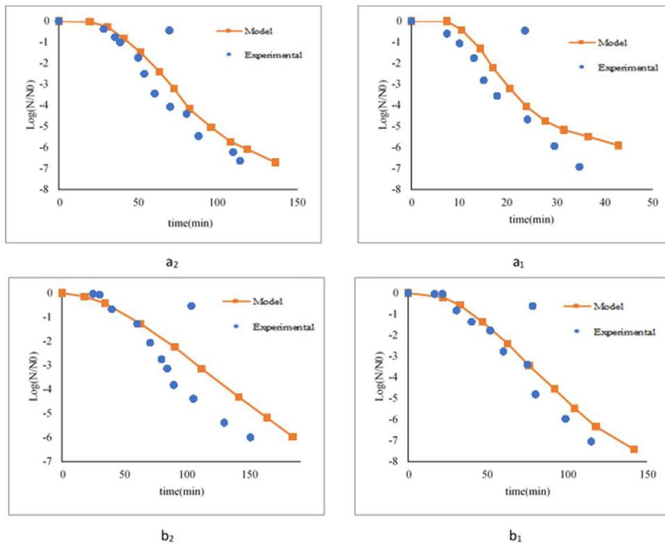
**Figure 6.** Prediction of *Listeria monocytogenes* inactivation curve using high-pressure supercritical fluid by the log-logistic model at 25 °C in (a) brine, (b) broth and pressures (1) 6.05 MPa, (2) 3.02 MPa.
