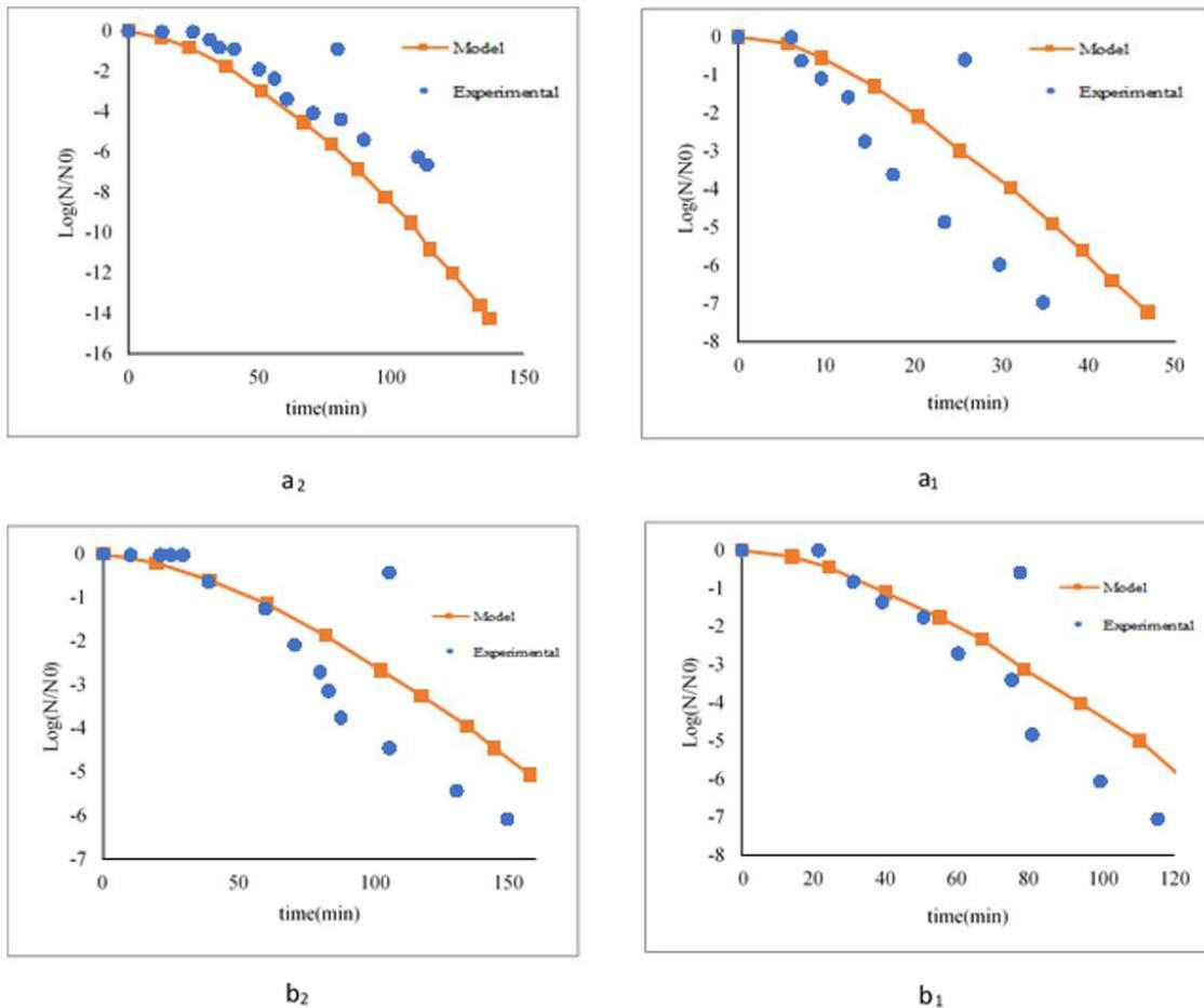
**Figure 3.** Prediction of *Listeria monocytogenes* inactivation curve in (a) saltwater, (b) broth, with the high-pressure supercritical fluid process at 25 °C by Weibull model and pressures (1) 6.05 MPa, (2) 3.02 MPa.
