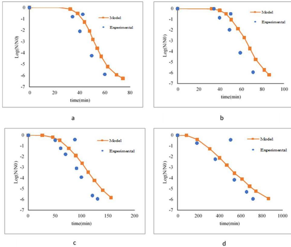
**Figure 5.** Prediction of *Saccharomyces* deactivation inertia curve using supercritical fluid at 40 °C and pressures of (a) 10 MPa, (b) 7.5 MPa, (c) 5 MPa, (d) 2.5 MPa.
