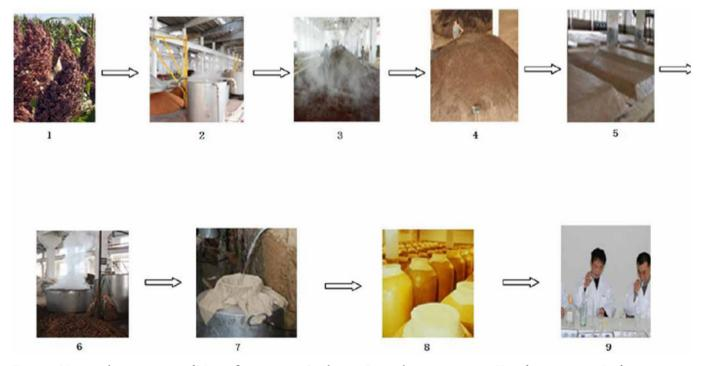
**Figure 1**. Main production process of Maotai flavor wine. 1. Sorghum 2. Steamed grain 3. Airing 4. Heap fermentation 5. Pit fermentation 6. Steamed wine 7. Take wine 8. Storage 9. Tick.
