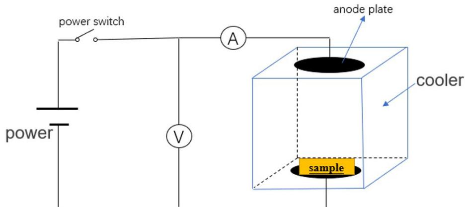
Figure 6. Schematic representation of a Electrostatic Field (EF) procedure.
