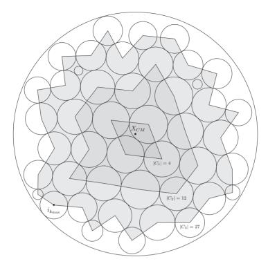
Figure 5 – A suboptimal solution: 45 circles inside the container.
