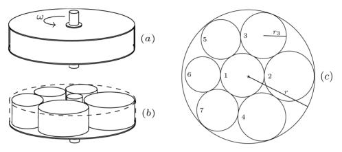
Figure 1 - Circular devices inside a rotating circular container and a feasible solution
