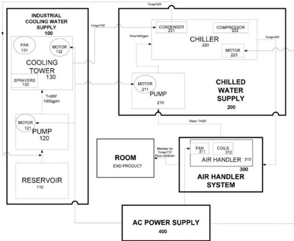
Figure 5 – Reliability block diagram of the HVAC (USDoD, 2006).
