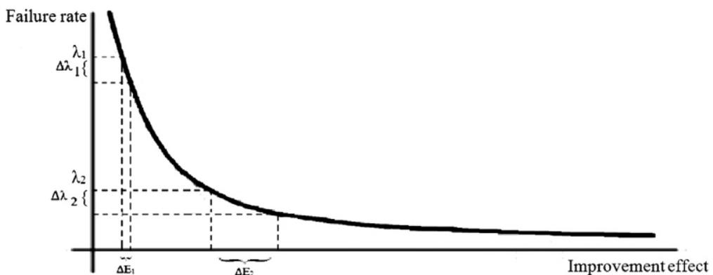
**Figure 1** – Nonlinear relation between failure rate and improvement effort.
