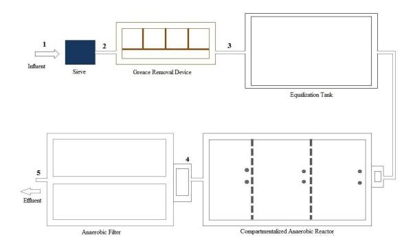
Figure 1. Schematic representation of the fish processing industry's effluent treatment plant and indication of sampling points (1 to 5).
