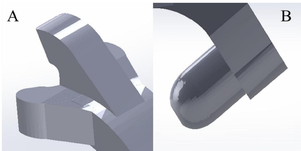
Figure 3. Basic components of the surgical guides: clamping component model lateral oblique views (A) and perforation guide component model in lateral views (B).
