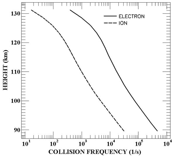
**Figure 3** – Vertical profile of the ion-neutral collision rate (dashed line) and vertical profile of the electron-neutral (continuous line) calculated for the RESCO radar site location, covering the range height from 90 to 130 km, during equinox, at 12 h (local time).
