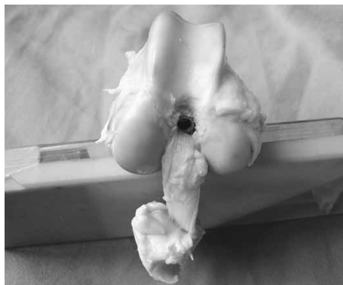
Figure 4 – Photograph of specimen fixed using interference screw.
