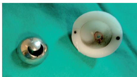
Fig. 8 - Fracturing of the cobalt-chrome femoral head (left) and polyethylene wear (right).
