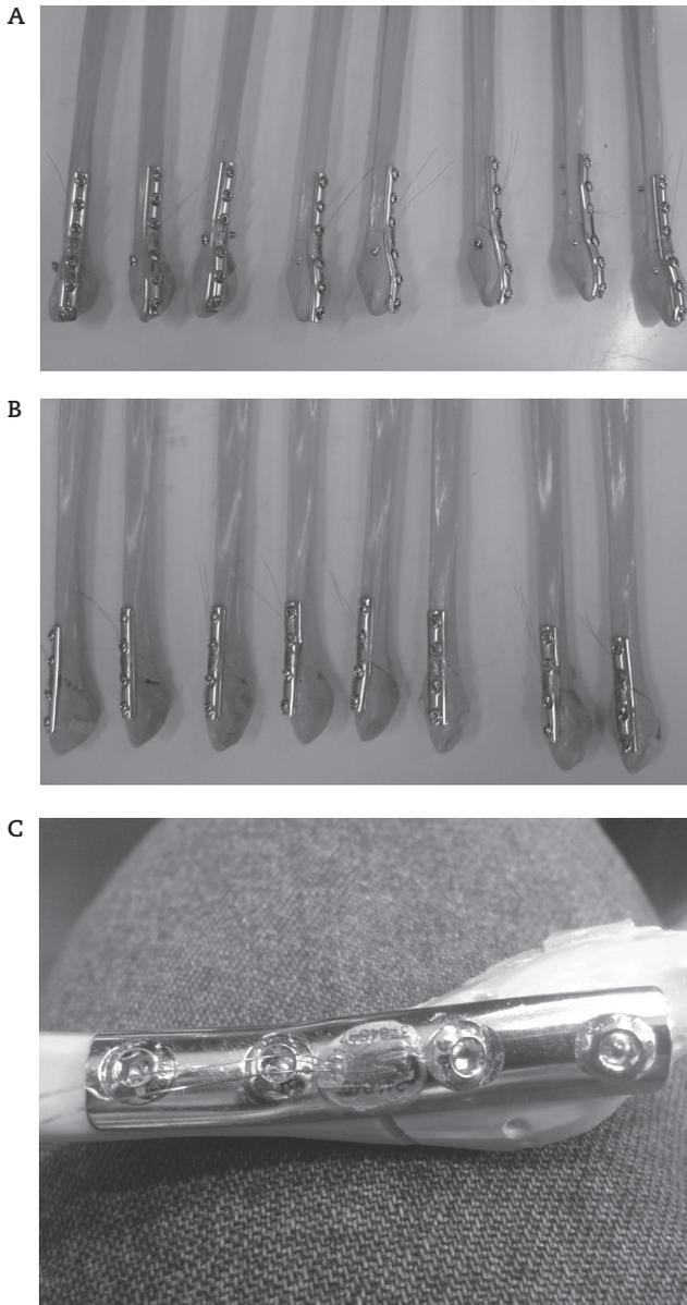
**Fig. 2 - Right synthetic fibulas. (A) fixation of a lateral plate with six holes. (B) fixation of a posterior plate with six holes. In both groups, it is possible to observe small electrodes fixed to the plates. (C) A strain gauge was used to measure the deformation in the center of the plates.**
