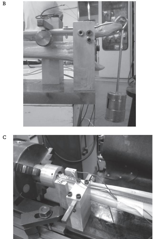
**Fig. 3 - Illustration of the trials. (A) equipment used for data acquisition and analysis. (B) weight applied to the fibula, with simulation of supination effort. (C) fibula inserted in the mandrel used to apply torsional forces.**
