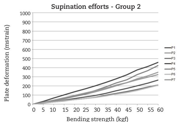
Figs. 5 and 6 - Deformation of Groups 1 and 2, respectively, in the first trial, due to the deforming strength in supination.
