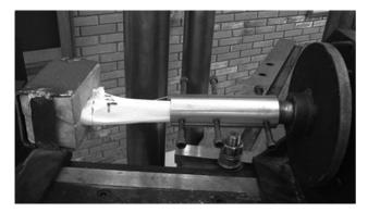
Fig. 5 Mechanism for the application of rotational loads.
