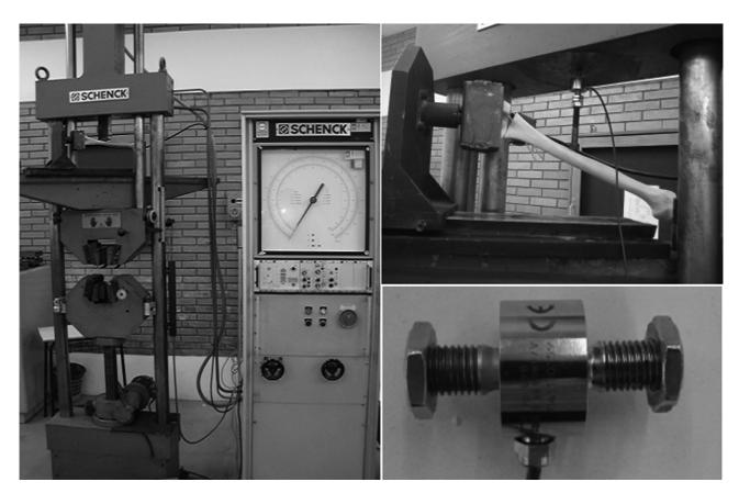
Fig. 3 Universal tensile testing machine model UPM 200 and an HBM U9B load cell (20 KN = 1 mV/V)
