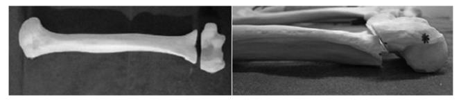
**Fig. 1** Test specimens: cross-section of a synthetic humerus at its distal portion, through the olecranon fossa at 3 centimeters from the distal edge of the bone, simulating a supracondylar fracture.
