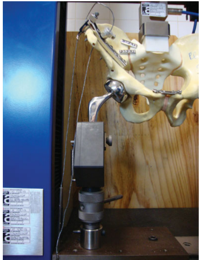
Fig. 4 The right iliac bone was connected to the lower head of the machine by means of two steel cables (diameter 1.6 mm) that simulated the gluteus medium muscle for pelvic stabilization. The cables were attached to the ilium with the aid of a plate. One of the cables was attached at the level of the iliac crest and the other to the anterior gluteal line, near the tubercle of the iliac crest.
