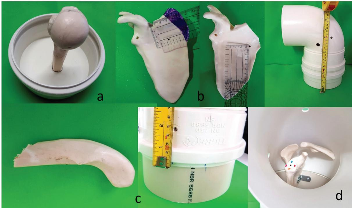
**Fig. 2** (A) Humeral fixation at the cap; (B) section of the scapula, hole for fixation and fixation point at the external structure; (C) clavicle section; (D) internal assembly.
