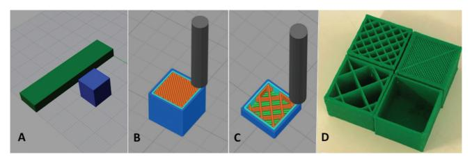
**Fig. 1** Computer images demonstrating the creation of study objects with 3D technology. A) square and rectangle drawing in CAD software; B) preparation of the object for 3D printing with internal filling (infill) of 100%; C) preparation of the object with partial internal filling (hollow); D) photography showing printed objects with different filling percentages. Source: authors' file.
