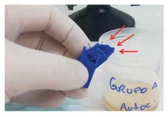
**Fig. 3** Photography demonstrating detail in the process of sowing hollow objects (NS), which were broken immediately before placement in Brian Heart Infusion (BHI) broth. Source: authors' file.
