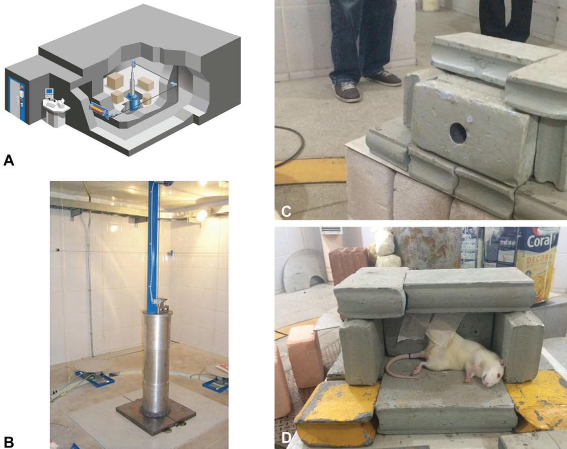
**Fig. 1** Method for irradiation. (A) 3D plan of the collimator room; (B) Cobalt 60 Source; (C) Lead blocks for directing the radioactive beam; (D) Anesthetized animal, positioned for procedure.
