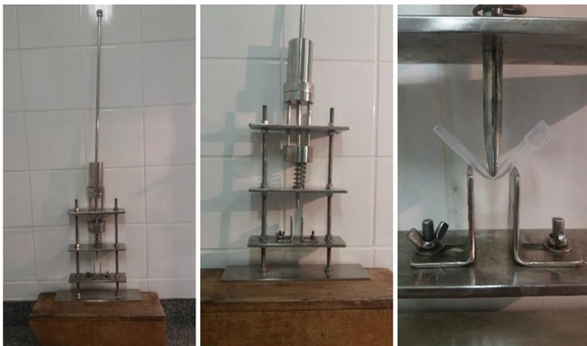
**Fig. 2** Guillotine developed for femoral diaphyseal fractures. On the left, the entire structure can be seen. In the center, a detail of the weight at the end of the track. On the right, the tip of the guillotine with a simulation of fracture production.
