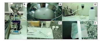
FIGURE 1 - Stages in the production of vegetable cellulose nanofibrils: A) Mass Colloider Masuko mill; B) cellulose suspension being processed by the mill; C) utensils used to produce nanofibrilated cellulose suspension; D) vacuum filtration for membrane production; E) translucent produced film.
