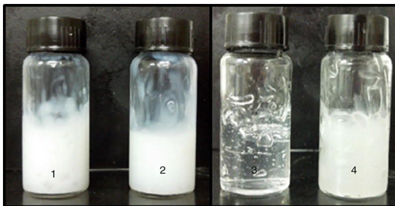
Fig. 1. Hydrophilic gels prepared with Carbopol® Ultrez 10 NF as gelling agent: (1) hydrogel with blank nanoparticles (HNP); (2) hydrogel with CcVO encapsulated in PLGA nanoparticles (HNPVO); (3) hydrogel blank (HB); (4) hydrogel prepared with free CcVO (HVO).
