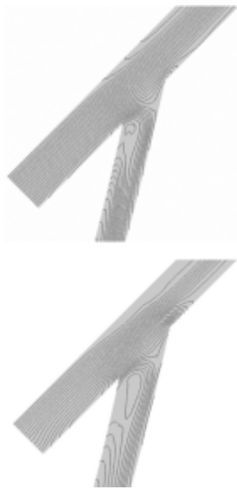
Fig. 9 - Behavior of the flow in the graft and pulmonary artery according to the diameter of the PTFE graft. Note that the recirculation region in the graft increases as the diameter of the graft increases
