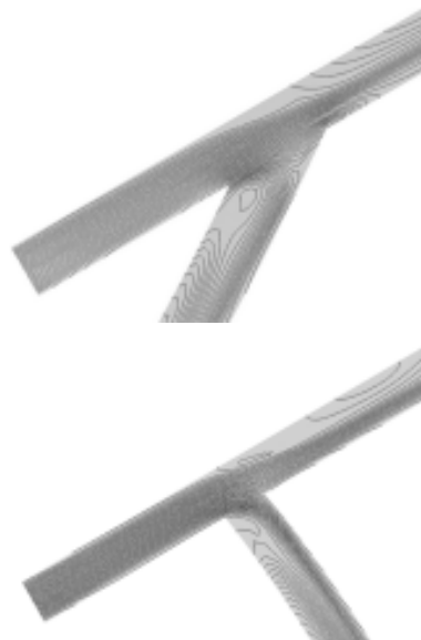
Fig. 10 - Lines of current for anastomosis of 30° and 90°. Near to the proximal anastomosis there is a region of low velocity and with recirculation, where the behavior of the flow in this region is favored by the greater angle of the graft
