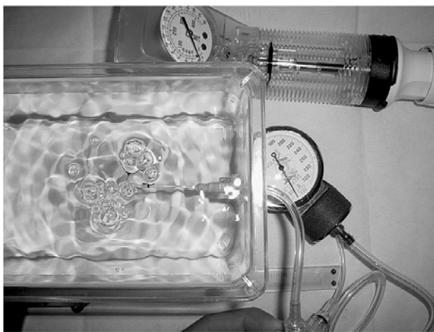
Fig. 5 - Arterial sample showing the moment of rupture and air leak
