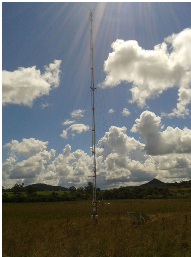
Figure 1 - Micrometeorological tower installed at the Santa Maria experimental site. Photography: personal collection of researcher Michel Stefanello (2017).
