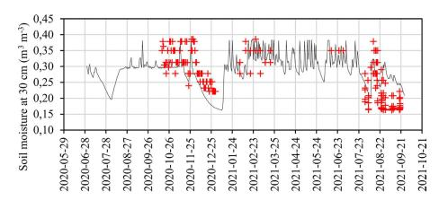
Fig. 3 - Variation of soil moisture from September 2020 to September 2021. Points represent measurements with tensiometers, and the line is the soil moisture simulated by a water balance.
