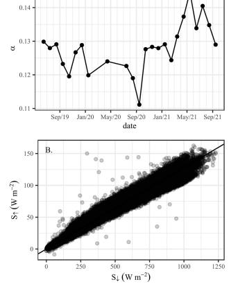
**Fig. 5** - Variation of albedo per month from June - 2019 until September - 2021. Points in figure A represent the slope of the regression analysis between  $S_1$  and  $S_1$  performed for each month.
