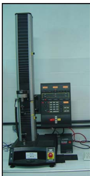
FIGURE 4 - Front view of the dynamical strain electromechanical test instrument (Instron 4443)
