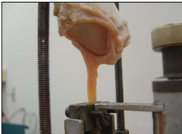
FIGURE 3 - Testing setup. Specimen sample type B fastened to the MTUE machine
