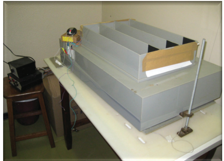
FIGURE 1 - Computed treadmill utilized for gait analysis.
