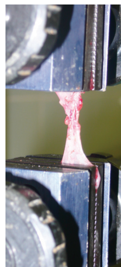
FIGURE 2 - Sample of the abdominal wall subjected to tension for measurement of tensile strength.
