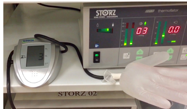
Figure 2 - Validation of semi-automatic manometer monitor for experimental use in rats. Latex glove insufflation after simultaneous adaptation to professional insufflator, that brought forth equivalent markings in pressure variations between 1 and 10mmHg. Equivalent measurements can be seen in both insufflator and sphygmomanometer monitors.
