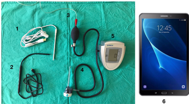
Figure 1 - Set of instruments adapted for laparoscopic surgery in rats. 1. Micro camera with rigid rod 5mm. 2. Micro camera with flexible rod 5.5mm. 3. Adaptation of CO 2 conductive tube. 4. Detail of the CO 2 tube connected to the 5mm trocar. 5. Semi-automatic manometer gauged. 6. Tablet Android 10.5\".
