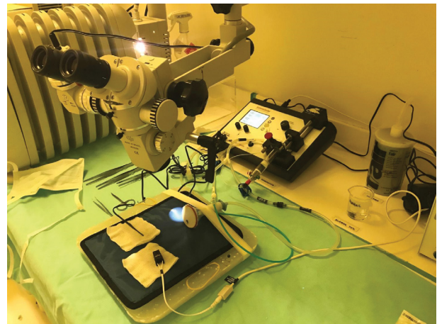
Figure 1 - Sommo Suite anesthetic equipment (small animal anesthesia system) of the rodents with a nasal mask and heated bed.
