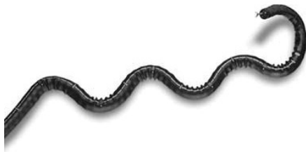
Figure 11 - Independent movable segments controlled by NeoGuide system. 35
