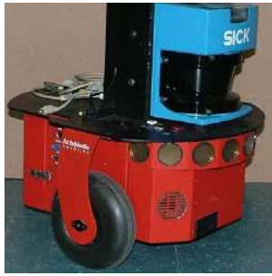
(a) The mobile robot used, with the onboard laser scanner.
