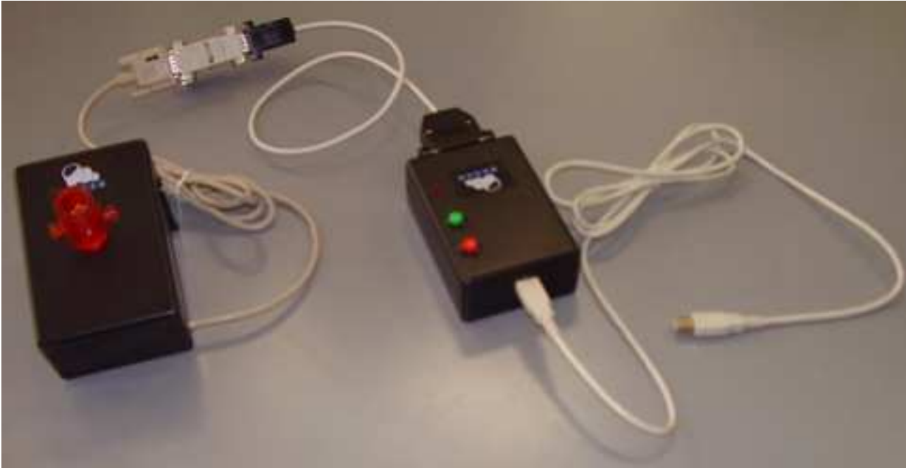
Figure 1: Digital manovacuumeter developed by NEPEB (Núcleo de Estudos e Pesquisa em Engenharia Biomédica). On the left, the pressure signal acquisition module; on the right, the A/D converter module.
