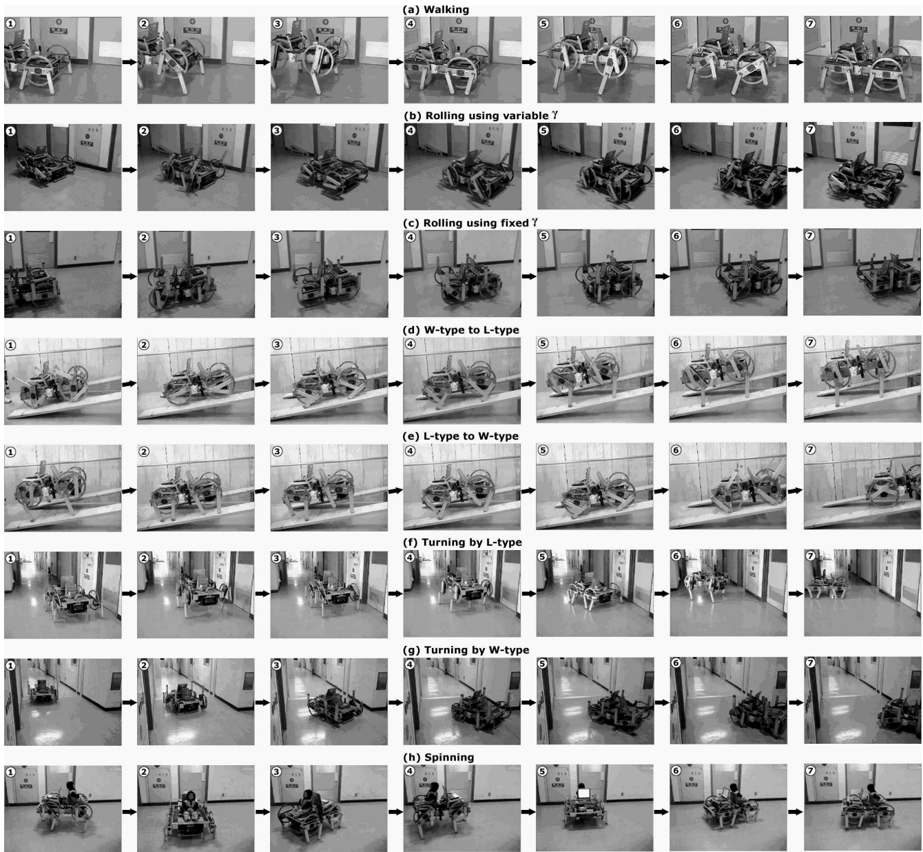
Figure 14: Experimental results in the walking, rolling using variable \gamma , rolling using fixed \gamma , switching from W-type to L-type, from L-type to W-type, turning by L-type, turning by W-type and spinning in (a), (b), (c), (d), (e), (f), (g) and (h), respectively.
