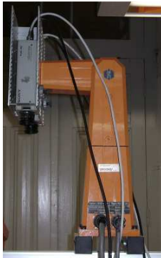
Figure 17: The vision system of Janus.
