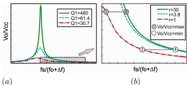
Figure 14: Operation region. (a) Gain curves. (b) Zoom of operation region.
