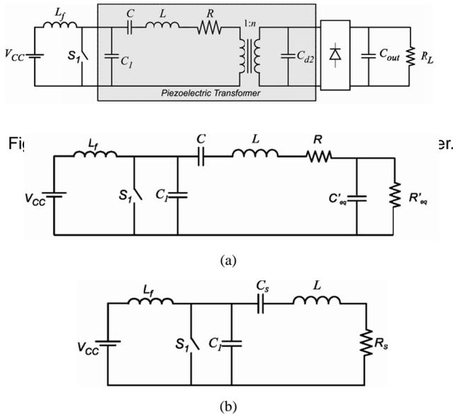
Figure 2: Simplified Class-E Converter. (a) Output elements in parallel arrangement. (b) Output elements in series arrangement.
