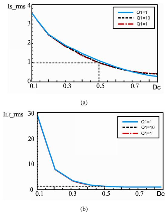
Figure 7: Rms current in the inductor and in the switch as a function of Dc and Q<sub>1</sub>. (a) Current in the switch. (b) Current in the inductor.
