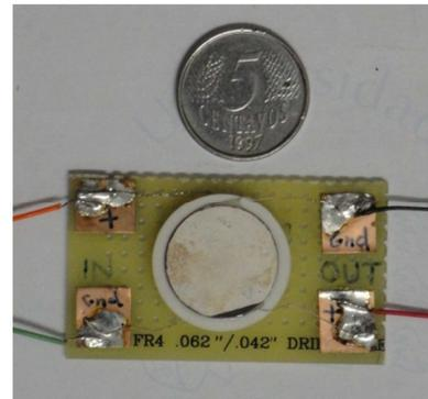
Figure 18: Piezoelectric transformer used for the implementation.
