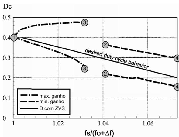
Figure 17: Desired duty cycle behavior.
