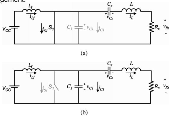
Figure 3: Stages of the converter at steady state. (a) Stage I - \$(t\_0 \leq t < t\_1 : DcT)\$. (b) Stage II - \$(t\_1 \leq t < t\_2 : (1-Dc)T)\$.
