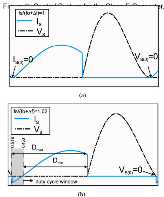
Figure 10: Current and voltage in the switch for different switching frequencies. (a) Nominal frequency. (b) Higher frequencies.
