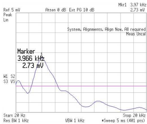
Figure 14: Representation of the microphone output signal for the tube without fouling (pipe with water).
