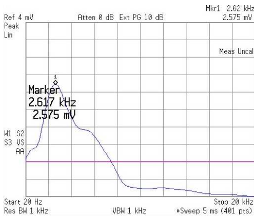
Figure 15: Representation of the microphone output signal for the tube with 5 mm of fouling (pipe with water).
