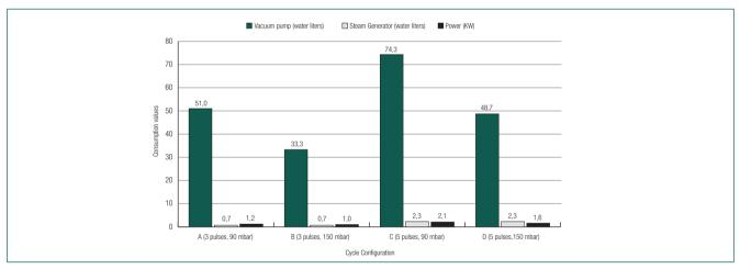
**Figure 1.** Average water and power consumption during the conditioning phase for each cycle configuration
