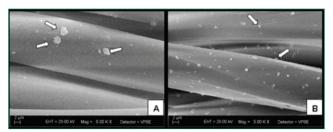
**Figure 2.** Electromicrographs (5000x) of the fabrics after passing the fluid plus the bacterial inoculum (*Staphylococcus aureus*). (A) irregular structures on the surface of the oxford fabric thread; (B) irregular structures on the surface of the microfiber fabric thread
