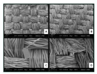
**Figure 1.** Topographic electromicrographs of oxford and microfiber fabrics. (A) panoramic view of the oxford fabric; (B) panoramic view of the microfiber fabric; (C) macropore in the region of intersection of the oxford fabric threads; (D) region of intersection of microfiber fabric threads
