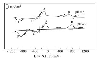
**Figure 1.** Typical cyclic voltammogram, obtained with an electrode of galena in an aqueous solution of KCl 0.1 M and  $3.37 \times 10^{-4}$  M potassium ethyl xanthate, at pH 8.0 and 9.0, with starting potential -280 mV (rest potential) and initial scan in the anodic direction. Sweep rate 10 mV/s.
