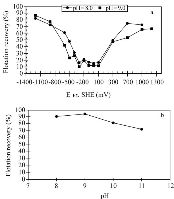
**Figure 3.** a: Influence of applied potentials on galena floatability in an aqueous solution of KCl and  $3.37 \times 10^{-4}$  M potassium ethyl xanthate. b: Influence of pH on the floatability of sphalerite in the same solution.
