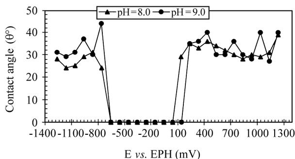
**Figure 2.** Contact angle measurements for galena at pH 8 and 9 under applied potentials from -1258 to 1242 mV, in an aqueous solution of KCl and 3.37 x 10<sup>-4</sup> M potassium ethyl xanthate.
