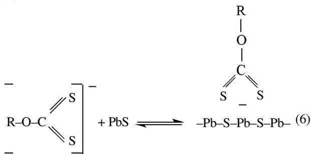
Under this condition, with sulfur in excess of lead, the surface becomes hydrophobic, which favors flotation.
