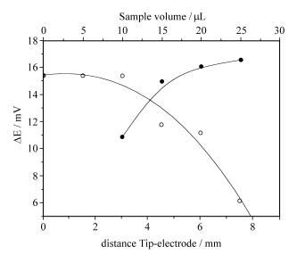
**Figure 2.** Influence of sample volume and electrode-tip distance upon potentiometric response. Concentration of sodium salicylate:  $1.0 \times 10^{-2}$  mol L<sup>-1</sup>. Effect of sample volume; Tip-electrode-distance: 0 mm; dispension rate: high. Effect of Tip- electrode distance. sample volume: 15 µL; dispension rate: high.
