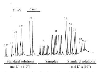
**Figure 3.** Batch injection calibration runs for standard sodium salycilate solutions and acetylsalycilic acid from tablet samples.From left to right duplicate signals from sodium salicylate standards (0.75, 1.0, 2.5, 5.0 and 7.5 x  $10^{-2}$  mol L<sup>-1</sup> of sodium salicylate solutions); replicate signals for tablet samples of acetylsalicylic acid; Standards in the reverse order.
