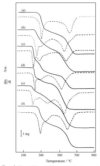
**Figure 3.** TG and DTG curves of the chemotherapic substances: (a) trimethoprim (7.216 mg); (b) sulfamethoxazole (7.943 mg); (c) ampicillim (7.593 mg); (d) tetracycline hydrochloride (7.706 mg); (e) rifampim (7.935 mg) and (f) trimethoprim-sulfamethoxazole (8.187 mg).
