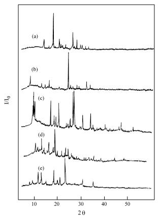
**Figure 2.** X-ray powder diffraction patterns of the chemotherapic substances: (a) trimethoprim; (b) sulfamethoxazole; (c) ampicillim; (d) tetracycline hydrochloride and (e) rifampim.
