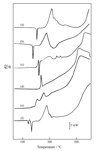
**Figure 4.** DSC curves of the chemotherapic substances: (a) trimethoprim (7.231 mg); (b) sulfamethoxazole (7.600 mg); (c) ampicillim (7.245 mg); (d) tetracycline hydrochloride (7.481 mg); (e) rifampim (7.551 mg) and (f) trimethoprim-sulfamethoxazole (7.840 mg).
