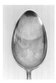
Figure 5. Silver spoon coated with TSHP. Just one half of the spoon was coated, while the other half remained uncoated. After this the spoon was immersed in  $H_2S$  saturated medium during 12 hours. Photo taken 8 months after the experiment.
