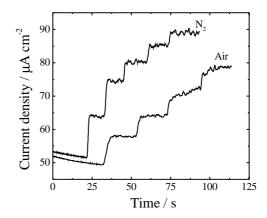
Figure 4. Amperometric response obtained at 0.65 V with the Ppy/GOx/ ferrocene biosensor in N<sub>2</sub> and air saturated buffer solutions. Each current step corresponds to an increase of 2 mmol  $L^{-1}$  in glucose concentration.
