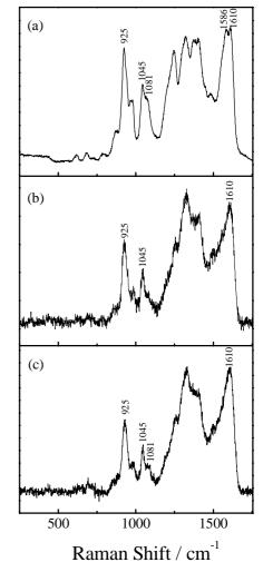
**Figure 1.** Raman spectra of (a) Polypyrrole film prepared from 0.1 mol L<sup>-1</sup> KCl aqueous solution, (b) Polypyrrole film formed from 0.1 mol L<sup>-1</sup> H<sub>2</sub>O/ ethanol solution, and (c) Polypyrrole/GOx/ferrocene film prepared from 0.1 mol L<sup>-1</sup> KCl + 0.003 mol L<sup>-1</sup> ferrocene + 10 mg mL<sup>-1</sup> GOx H<sub>2</sub>O/ ethanol suspension.
