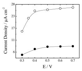
**Figure 2.** Effect of the applied potential on the current response of  $(\bullet)$  Ppy/GOx and (O) Ppy/GOx/ferrocene biosensors in 5.6 mmol L<sup>-1</sup> glucose in buffered (pH=7.0) solution, saturated with air.
