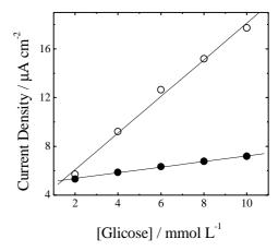
Figure 3. Calibration plots for glucose obtained for ( $\bullet$ ) Ppy/GOx measured at 0.65 V and (O) Ppy/GOx/ferrocene measured at 0.4 V in stirred buffered (pH=7.0) solutions, saturated with air.
