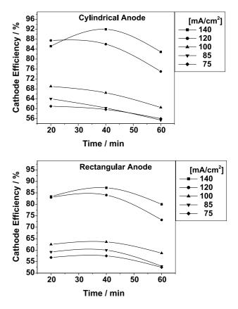
**Figure 3.** Effect of cathode current density on cathode current efficiency. The deposition realized with bath composition as in Table 1, bath temperature 80°C and cathode rotation rate 15 rpm.
