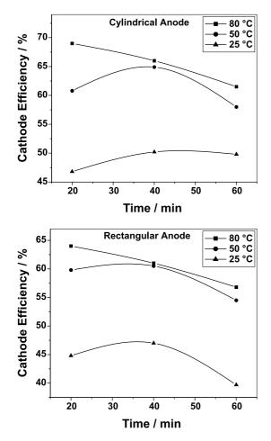
**Figure 2.** Effect of the bath temperature on cathode current efficiency. The deposition realized with bath composition as in Table 1, cathode current density  $100~\text{mA}~\text{cm}^{-2}$  and cathode rotation rate 15 rpm.
