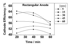
**Figure 1.** Effect of cathode rotation rate on cathode current efficiency. The deposition realized with bath composition as in Table 1, bath temperature  $80^{\circ}$ C and cathode current density  $100 \text{ mA cm}^{-2}$ .
