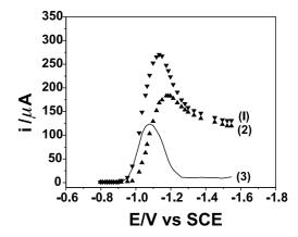
**Figure 6.** Squarewave voltammogram of bath solution of Table 1 at pH 9.5.  $\Delta E_s = 10$  mV,  $E_{sw} = 50$  mV, f = 100 Hz, conditioning potential -0.8 V, number of scans averaged 10. (1) forward, (2) inverse, (3) net current.
