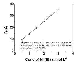
**Figure 7.** Concentration of Ni(II) versus squarewave net-current peak height. (○) experimental points, and (—) linear regression.
