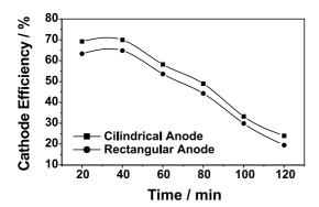
**Figure 4.** Effect of anode geometry on cathode current efficiency. The deposition realized with bath composition as in Table 1, bath temperature 80°C, cathode current density 100 mA cm<sup>-2</sup> and cathode rotation rate 15 rpm.
